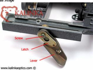
Step 1&2: Locate the retaining clip that is holding the lever onto the scope. Place a small flat screwdriver blade on the edge of the retaining clip, and using your thumb rotate the retainer out of its indentation. Once the retaining clip is rotated 90 degrees, you can easily slide it off of the center shaft of the clamp lever. It will now pull off of the scope.
