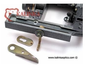
Step 4: Slide the scope onto your side rail and then reposition the lever so that you have a nice tight fit. Be careful not to over-tighten!
