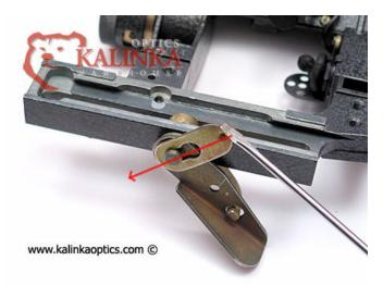
Step 3: Once the clip is removed, you can disengage the lever from its gear on the center shaft. Be sure not to lose the clip or the washer underneath the lever.
