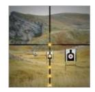
The SMART BDC™ reticle is factory set for 5.56/.308 and provides hold points for targets out to 500 yards.
